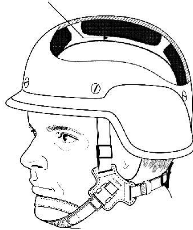
Figure 19. Crown Pad Not Touching Head
